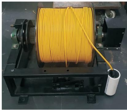
IGIS has introduced BHC-1 is a very handy device to quickly check the video capturing of bore well with clear vision of formation and strata of soil underneath with respect to its level in the open-wells and in bore-wells.
